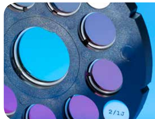
Test disc with colour-stable glass standards
