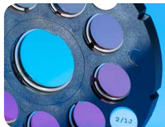
Test disc with colour-stable glass standards
